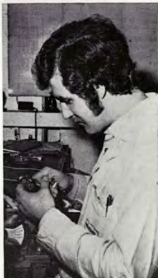
▶ The latest "I.T.T." mobile radio telephone being put through field tests on the new-band frequencies to the base at Newton Firs. The man doing the testing is Brian Nield, our telecommunications development engineer.
