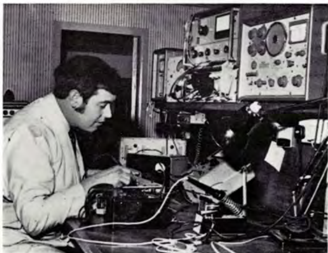
◀ Telecommunications foreman Mike Lewis at work in the Technical Workshop repairing a VHF mobile radio telephone, surrounded by a mass of electronic equipment.
