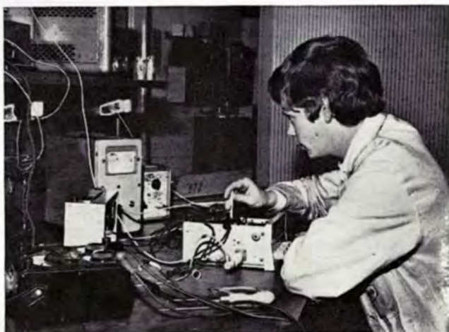
Instrument inspector, Dave Watts working on a converter on an Ultra set to allow vehicle battery polarity to be changed. ▶
